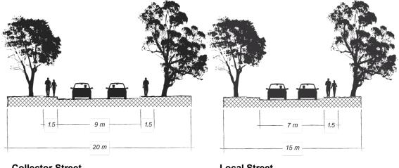
Collector Street Street Right-of-Way: Street Width: Minimum Sidewalk Width: Number of Sidewalks:
