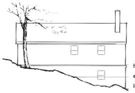
highest elevation established grade lowest elevation
